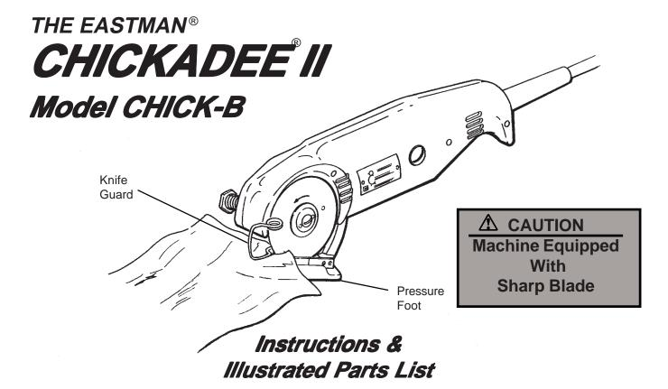
Your new Chickadee II is designed to replace hand held shears for increased performance and capacity with a minimum of maintenance and service. Equipped with either a round blade for general use or hexagonal blade for sheer or difficult to cut cloth. The Chickadee features a totally enclosed sharpener for fast and safe sharpening.
